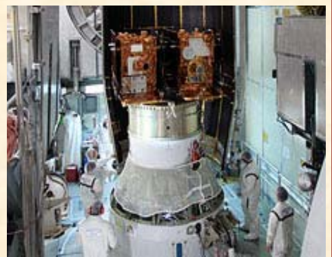
Image: The payload fairing is added to the GRail booster. Credit: NASA/KSC
